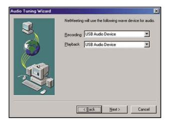
Here you can select the audio device for input/output. Please select the K1000A device (USB Audio Device in Windows 98/2000) and click Next. 4. On the next two screens you can adjust volume for playback and recording.
